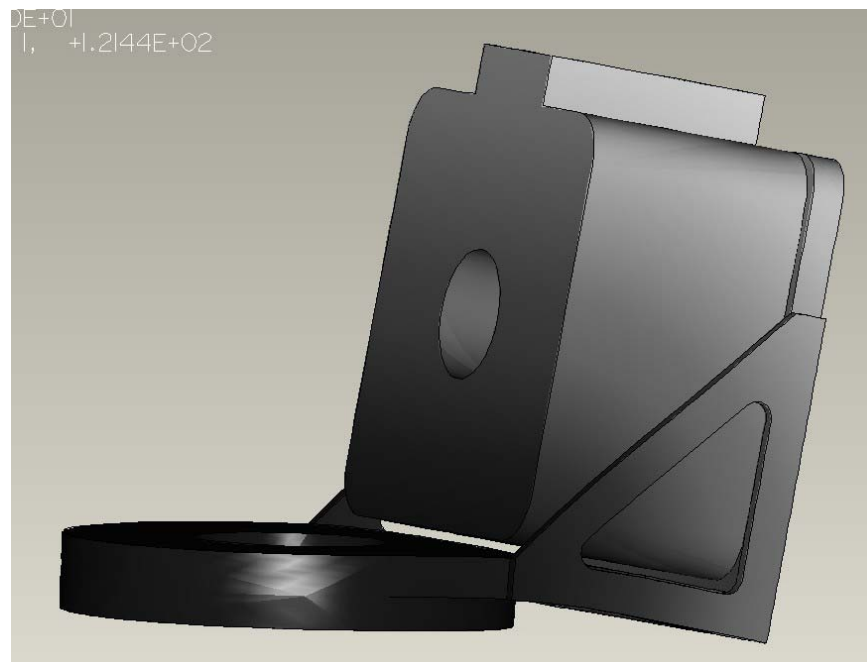
Figure 4: Final bracket design showing the deformation due to the static load. This is also the first mode shape for the modal analysis. The mass is 4.9 kg while the static stiffness is 10.6 \text{ N}/\mu\text{m} and the first natural frequency is 120 Hz.
